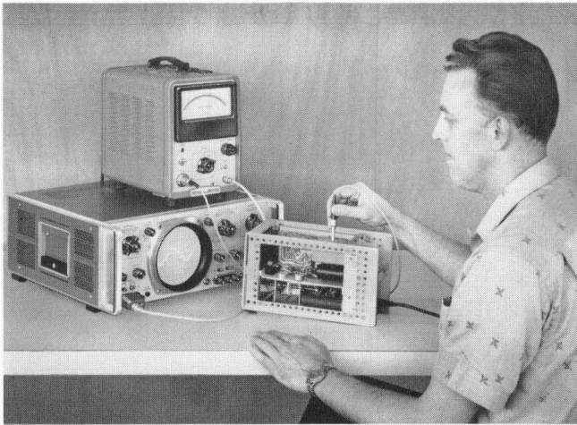
Fig. 2. Magnetometer probe being used to "sniff" external field from transformer. Waveform of ac field is displayed and measured on scope. DC fields are measured on -hp- 428B Milliammeter (upper unit).
